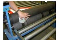
Microprismatic sheetings must not be overlapped a butt joint is the correct method.
