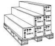
Nikkalite® boxed inks should be stored at a temperature of 15°C to 25°C in a metal cabinet preferably in the print shop 24 hours before use to acclimatise.
